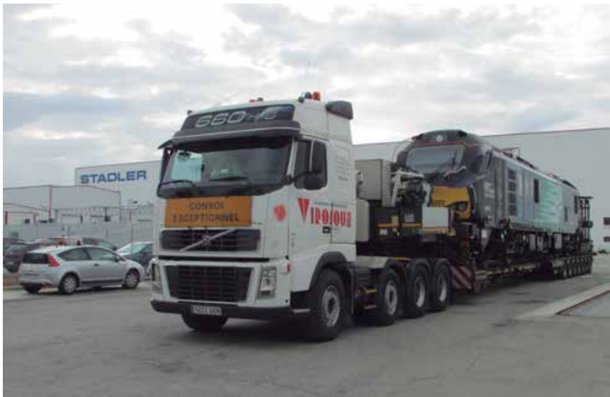
in passenger and freight transport services in the UK, at speeds up to 160km/h, combining both 25kV electric and diesel operating modes. Class 88 is a true dual-mode 4-axle locomotive adapted to UK gauge, with AC/ AC transmission and low
