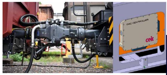
gon On Board Unit systems. With these telematic systems distributed in the wagons, the composition of the train is provided and its integrity is ensured, among other functions. On the other hand, the Digital Automatic Coupler
